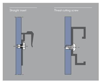
Remaining panel thickness: at least 2.5 mm. Anchoring depth: total panel thickness minus 3 mm.
